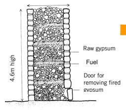
Figure 6: A Continuously fed vertical shaft kiln is an efficient way of processing large amounts of gypsum.
