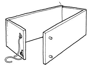
Figure 1: Mould for making gypsum plaster wall blocks
