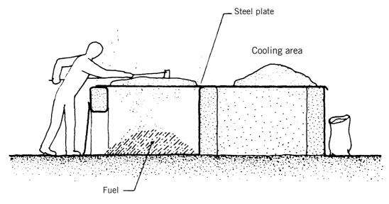
Figure 2: One simple production method is to heat the gypsum on a flat metal plate above a kiln
