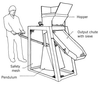
Figure 3: Crushing the gypsum ensures a more uniform product which requires less energy to heat. (This clay crusher was designed by J M Parry Associates Ltd.)
